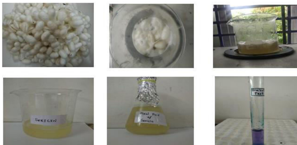
Fig: 3 Diagrammatic representation of extraction, purification, isolation and characterization of Sericin from silk waste cocoons
