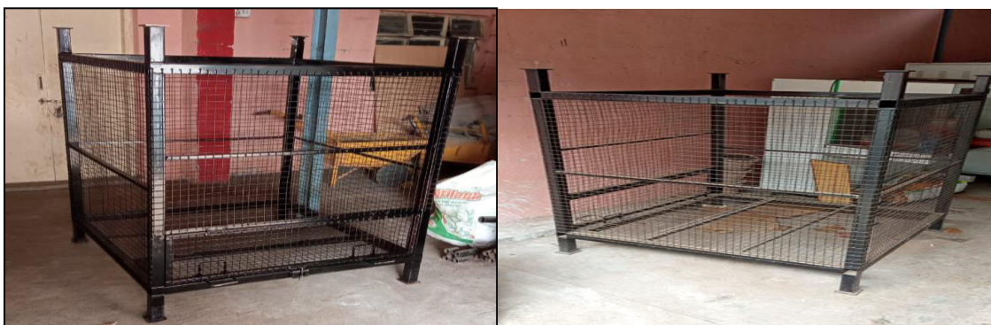
Fig 3.2: Stacking system Manufactured model for 1MT
