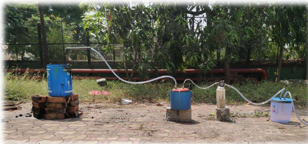
Fig. 1 Experimental set-up for pyrolysis process
