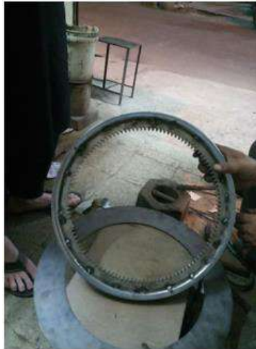
Fig.1: Internal Gear mounted on inner diameter of rim.
