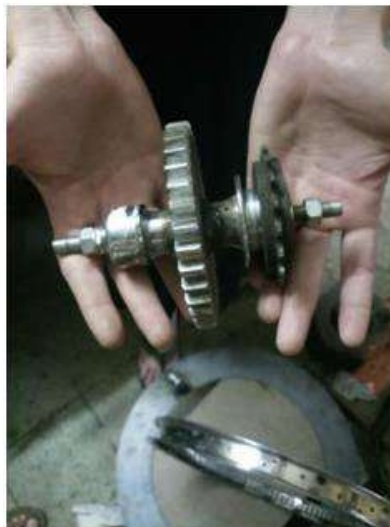
Fig.2: Spur Gear mounted on the hub.
