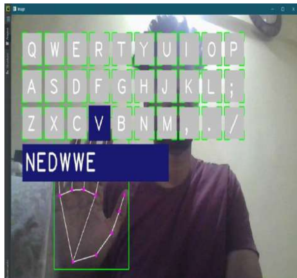
Figure 3: displays a live demonstration of typing using fingertip
