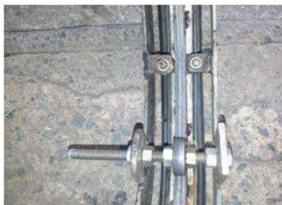
Fig.6: Support bearing mounted on M.S ring through nut and bolt and side bearing mounted on ring though nut and bolt.
