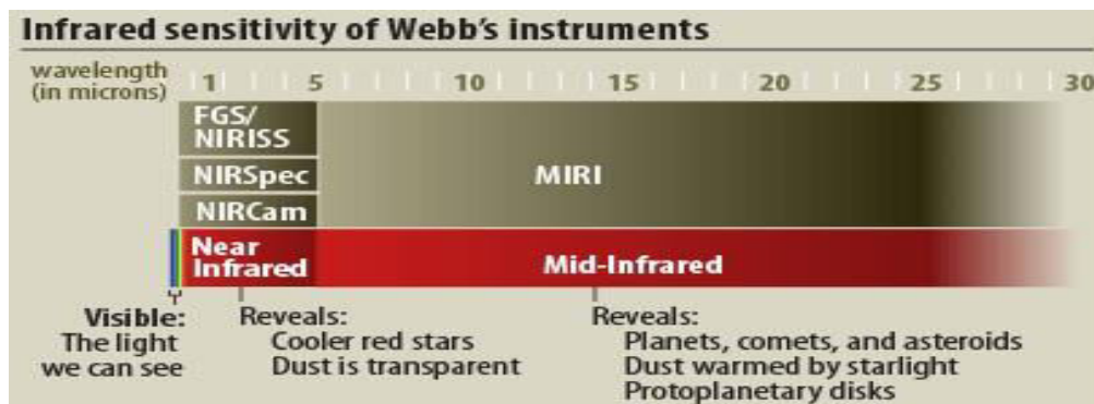
Fig 2.5:- range scale of NIRCAM (0.6 – 5 microns)
