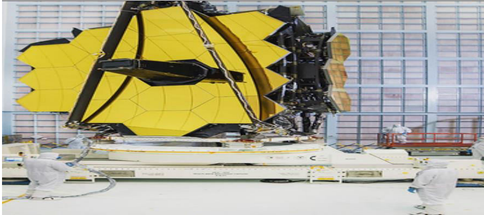
Fig 1.4:- hexagonal mirror of webb
