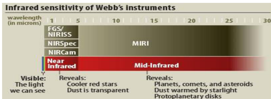
Fig 2.3:- range scale of NIRSpec ( 0.6 – 5 microns)
