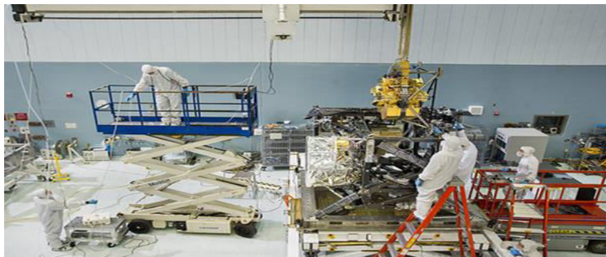
Fig 2.6:- NIRCam being installed into the instrument module
