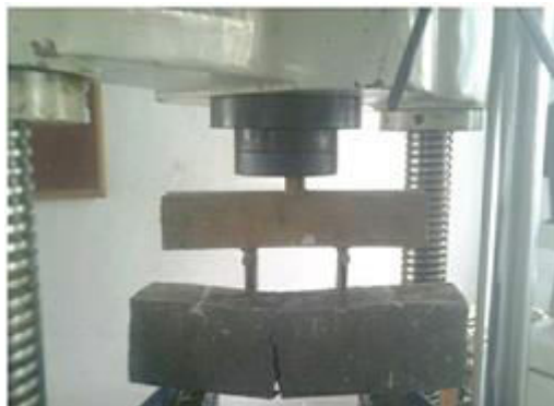
Fig 6: Flexural Strength Test setup – Failure mode of beam under
