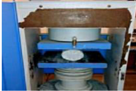
Fig.5: Cylinder split tensile strength test setup
