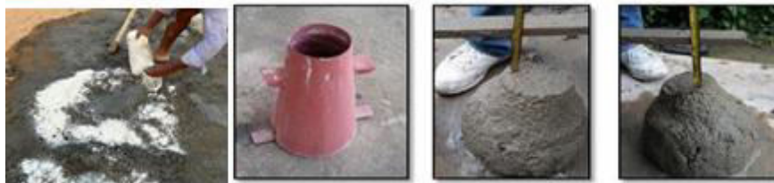
Fig.2: Concrete mixing with fiber and slump cone test
