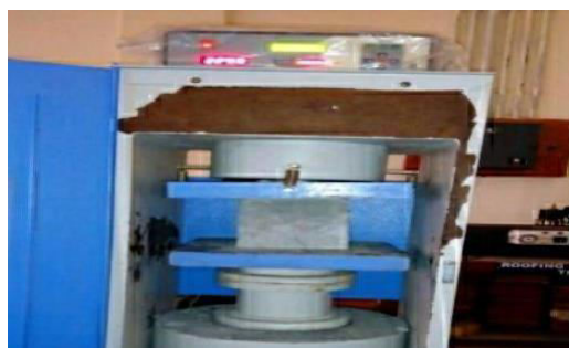
Fig.4: Cube Compression strength test setup
