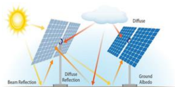
Figure 3: Albedo falling on Rear Surface
