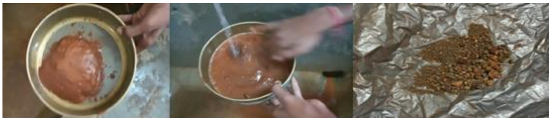
Figure 1: Paste of soil sample soaked in water, Separation of particles by flow of water and oven dried soil sample
