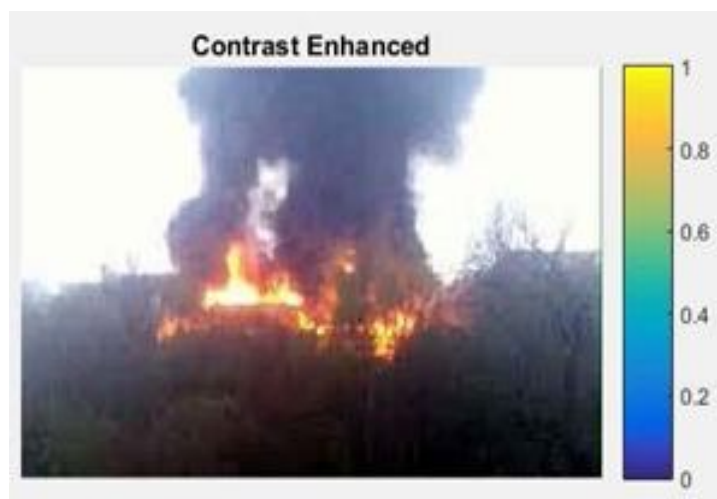
Figure 5. Contrasted Enhanced Image by previously proposed system [4] The enhancement level is poor and not effective for real time fire detection. It does not increase the fire color intensity through which it can be detected with high level of accuracy.
