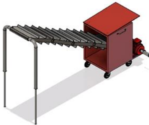
Fig.1 3D Model of a proposed Conveyor system for small scale industries
