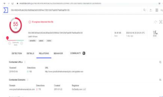
Fig 9: RELATIONS tab: The above shot shows which IP addresses, url's and domains have been checked to identify and detect the malware.
