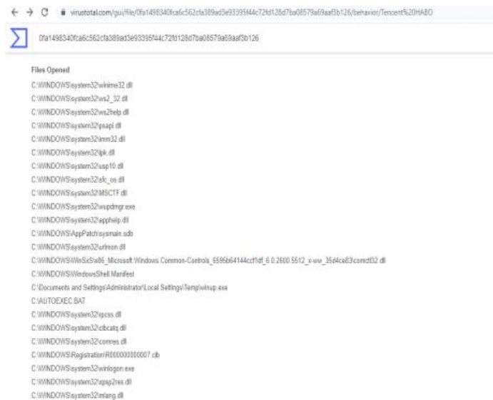
Fig 13: File System Actions: shows the files that are opened. These actions refer to those that are executed on the file system of the sandbox environment.
