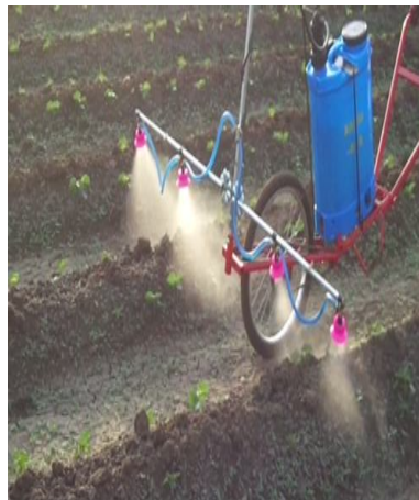
Figure 2: Working of Agrochemical Sprayer
