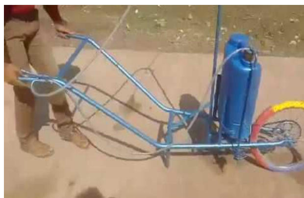
Fig. 5. Figure 3: Agrochemical sprayer trolley
