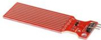
Fig. 5: water level sensor
