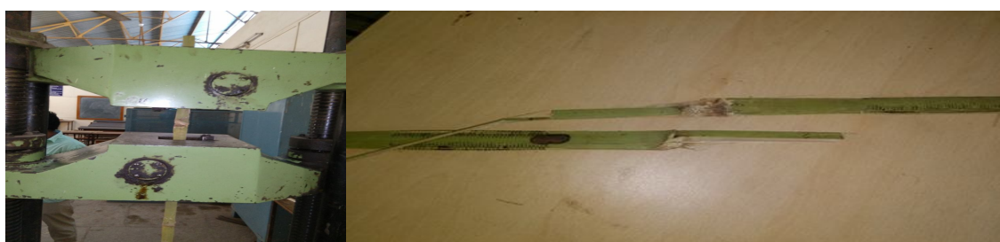
Fig.3 Tension test setup and failure pattern of bamboo sample
