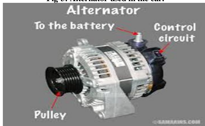
Fig-3: Alternator used in the car.
