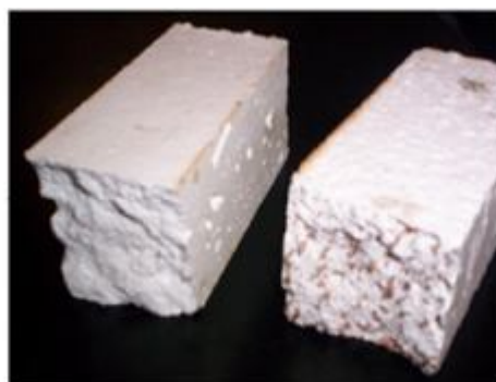
Fig. 1 – Gypsum plasters with cellulose fibres and cork
