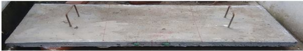
Marking of Demec Gauge Pellets
