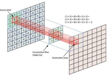
Figure-2: A kernel analysing an arbitrary picture [7]
