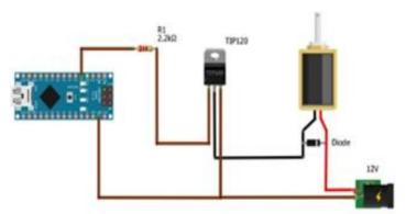
Figure-4: Interfacing of Solenoid with Node MCU
