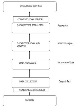
Fig-3.1: Architecture for city smart implementation using IoT
