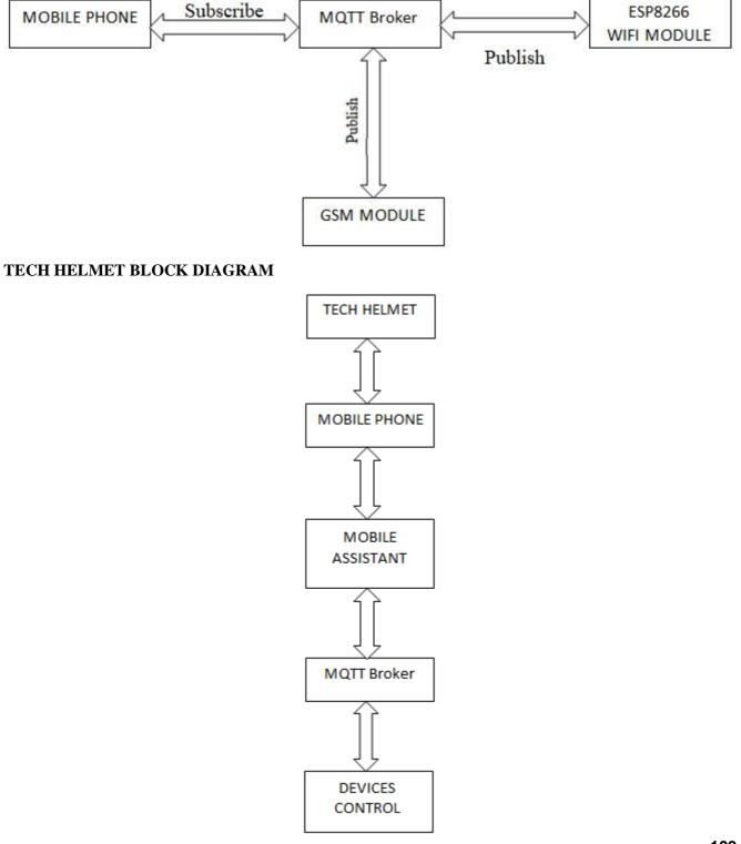
Hence the Helmet made to bring the various cross platform devices control through the voice of the user by its Text-to-Speech voice recognition system.
