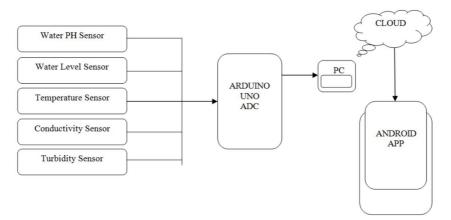
Figure-[1]: The illustration of smart water quality monitoring system in IOT environment [6]
