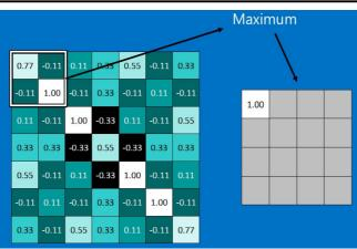
Figure-3: Max Pooling [8]
