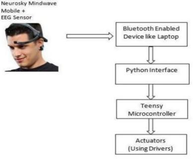
Figure-3: Block Diagram of Smart Robotic Gripper [2]
