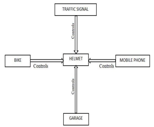
The helmet Integrates the Vehicle ,Mobile phone and Garage Devices through Mqtt server together were each devices can communicate with each other through the Mqtt broker with subscribe and publish protocol it is use full for M2M(machine-to-machine) communication.
