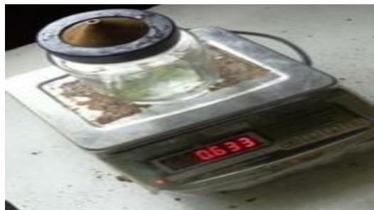
Fig-2: Pyconometer Apparatus in Specific Gravity Test
