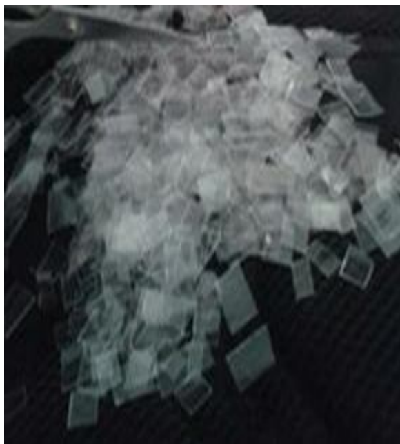
FIG-1: PREPARATION OF PLASTIC FIBERS FROM WASTE PLASTIC
