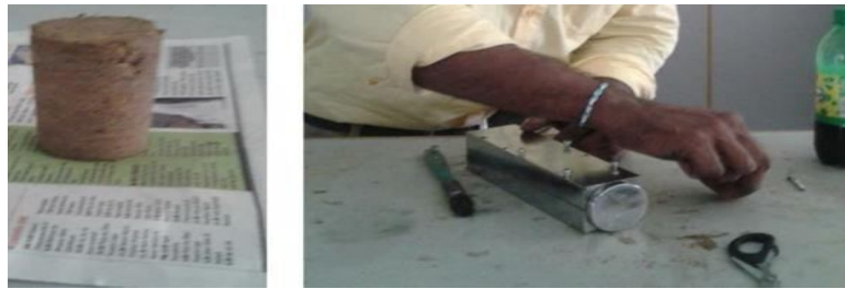
FIG – 10: UNCONFINED COMPRESSION TEST SAMPLE AND MOULD UNREINFORCED SOIL
