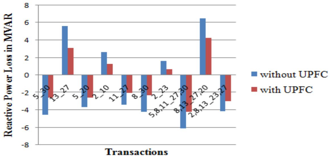
Figure-4: Reactive Power Loss for IEEE-30 bus system without and with UPFC devices
