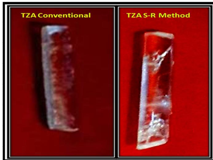
Fig – 1: Conventionally & S-R method grown TZA crystal
