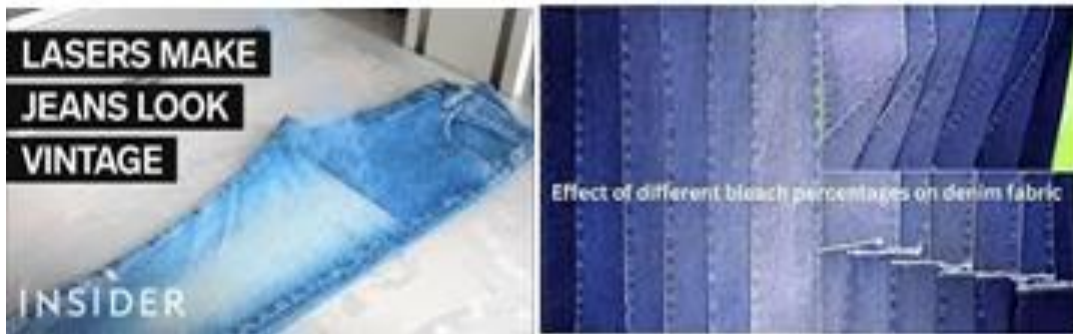
Fig. 2 Bleaching and Vintage effect, directly on textile and simultaneously with cutting
