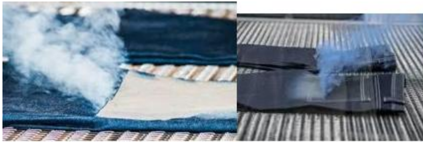
Fig. 1 Process of LASER Marking on Fabric
