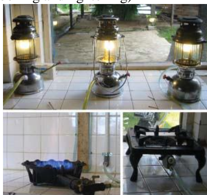
Figure 3. Utilization of biogas for mantle lamp and gas stove
